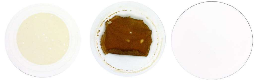
Figure 3: Filter appearance after passage of 100 ml oil sample with corresponding sediment concentration.
